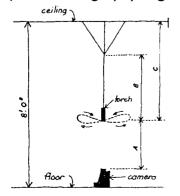
Making a physiograph: A is the distance between camera lens and the light bulb of the swinging torch; B is the distance between the light bulb and the point in the string at which side strings are fixed; C is the distance between light bulb and ceiling. The relation between B and C sets the pattern of the physiograph.
